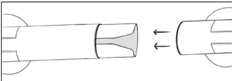
1 - Rod Splice/Connector should be inserted halfway into first rod, then insert remaining into the second rod.
