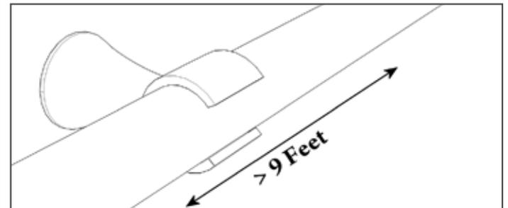
1 - Attach brackets to surface with 3 inch screw using appropriate type (drywall, wood, metal, concrete, etc.)
